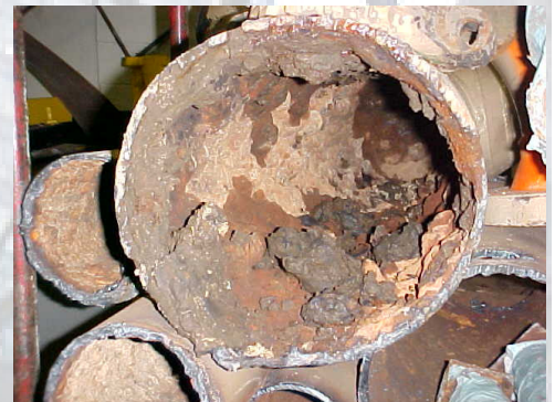
Below, the interior of the old piping showed signs of sediment build-up and corrosion.
